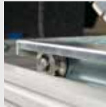
saw trolley with metal wheels
