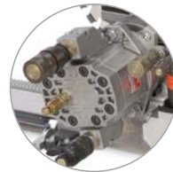
Main motor with leak-oil connection
